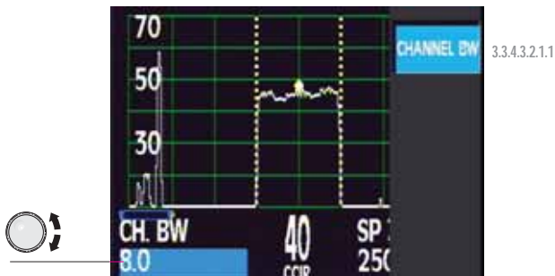
Figure 105.- Bandwidth of the digital channel
