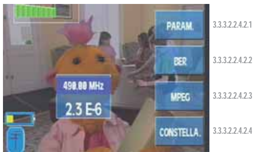
Figura 86.- MPEG decoding of a QAM channel
