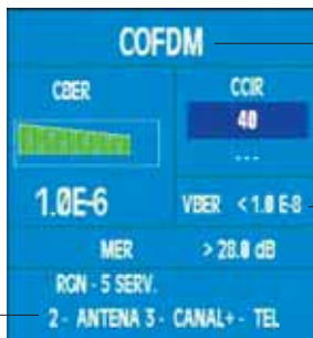
Figure 76.- BER measurement window
