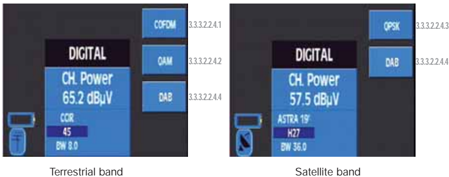
Figure 75.- Options for the BER measurements
