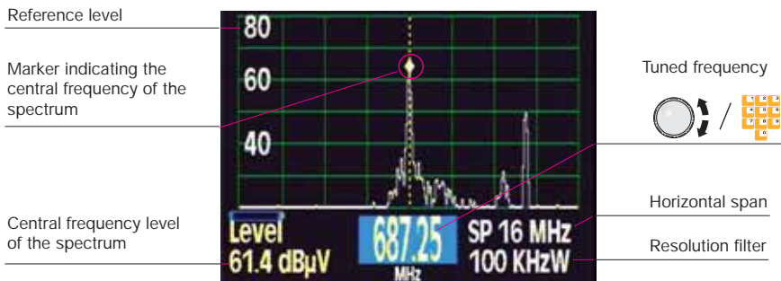
Figure 96.- Spectrum analyzer mode. Frequency tuning (analogue channel)
