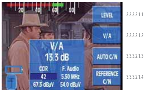
Figure 64.- Indication of V/A using the bars
