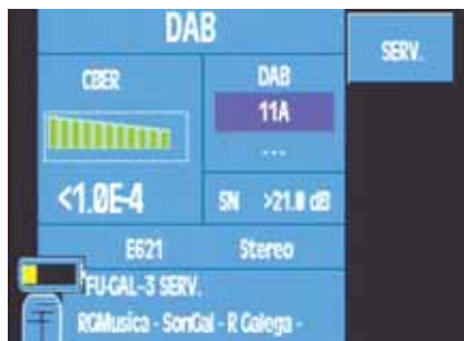
Figure 89.- Information on the DAB measurements
