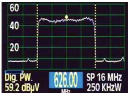
Figure 104.- Power of a digital channel
